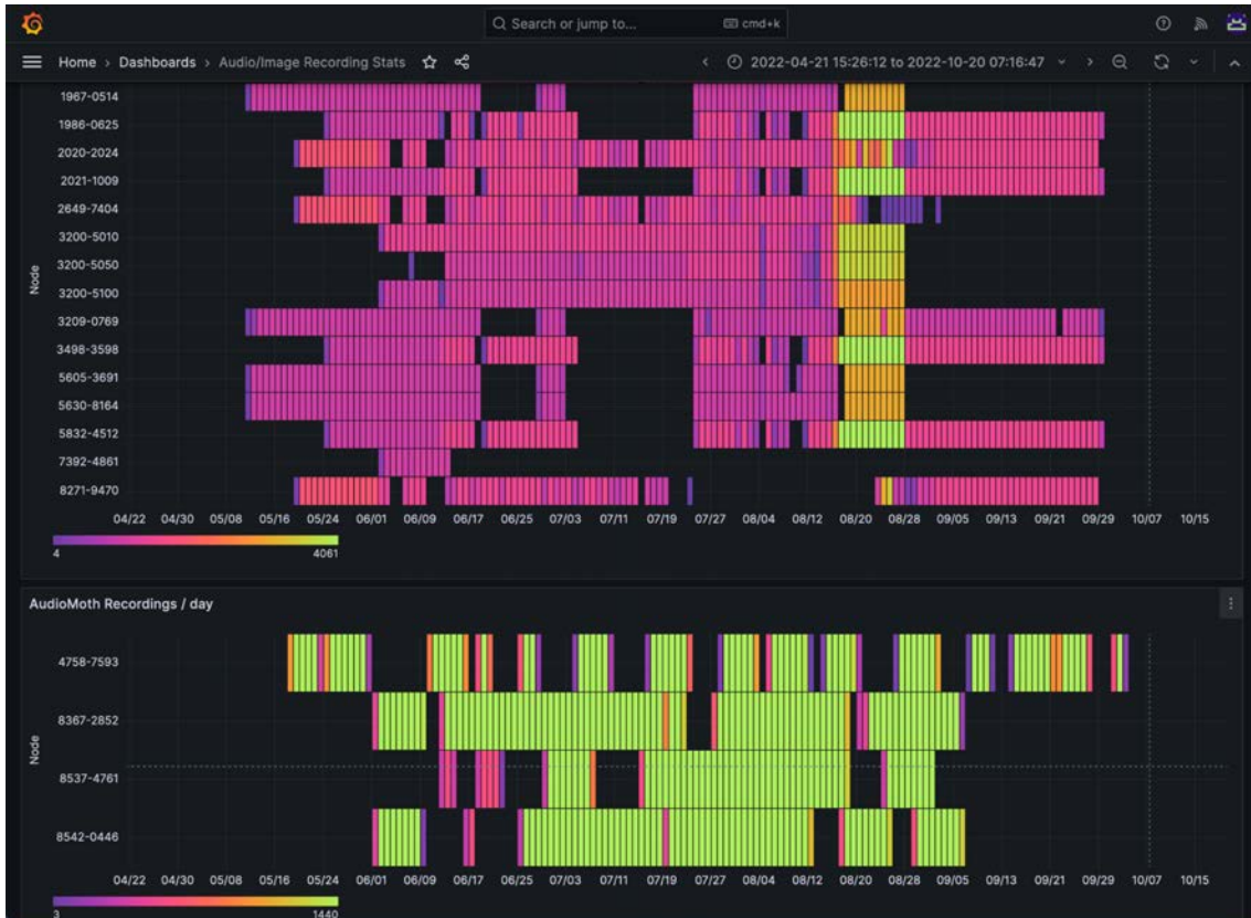
Fig. 4: A dashboard provides an overview of the stored audio and image files per sensor node and time interval and visualizes the amount of data using a spectral color code.
